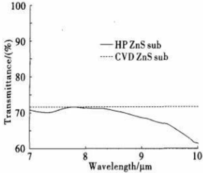
2. Transmission of Hot-pressed ZnS domes with AR/AR coating
